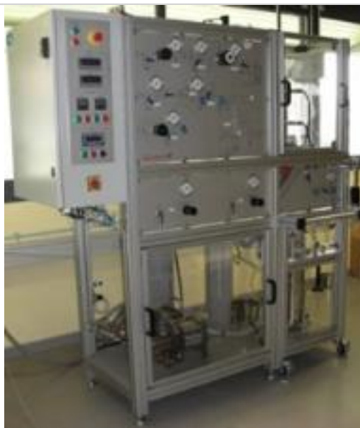
Sulfur balance cell
